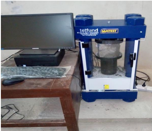
Plate 4: Placing the Concrete Cube in the UTM
