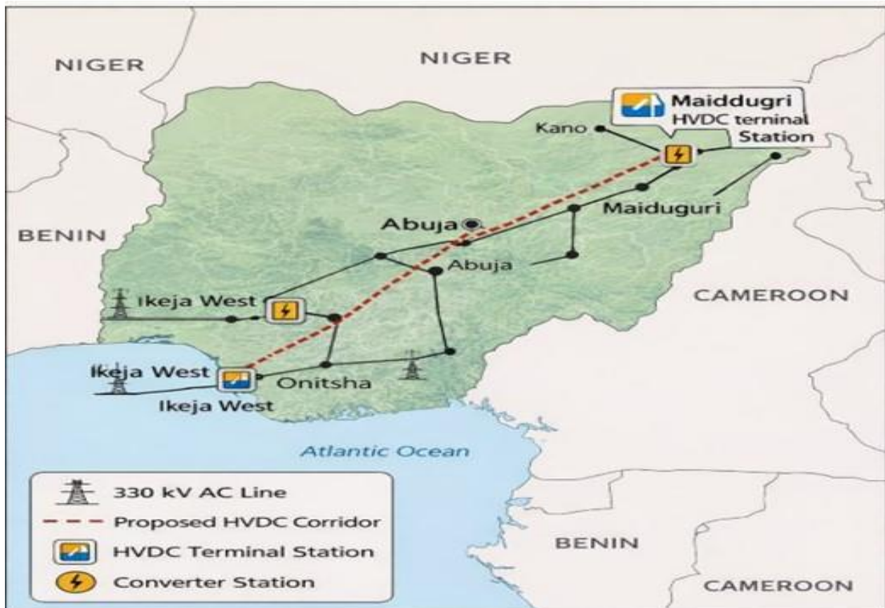
Figure 2: North-South Conceptual Representation of HVDC Integration into the Nigerian 330 kV Grid
