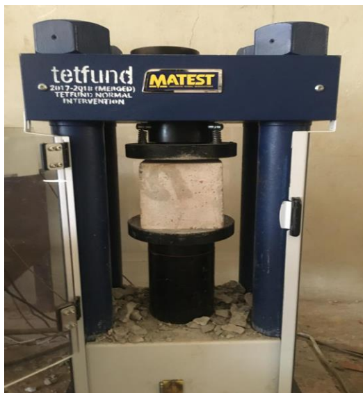
Figure 5: Compressive Strength Test
